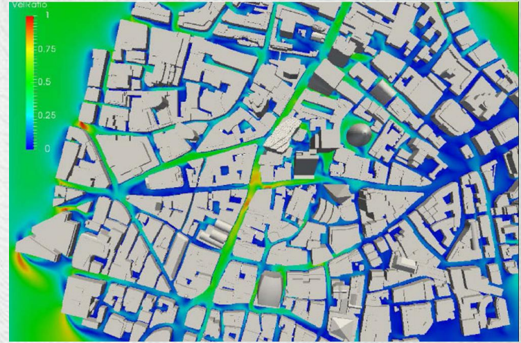
CFD simulation of London, UK microclimate 2016
